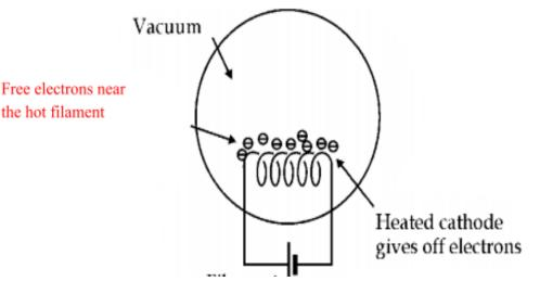
Heated filament gives out electrons
